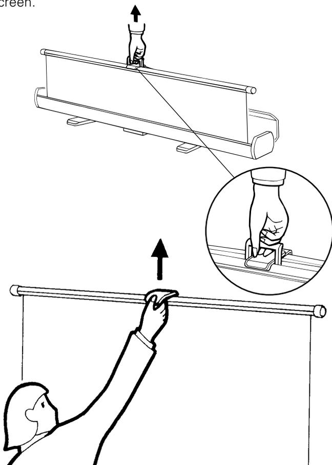
4. Place the end of the extending handle under the slat handle as shown below and raise screen to desired height. (100" model only)
