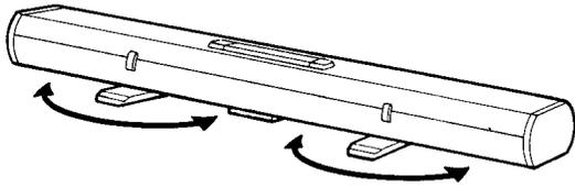
2. Release the latches and open the case cover. On the 90" and 100" models remove extending handle and extend it as shown.
