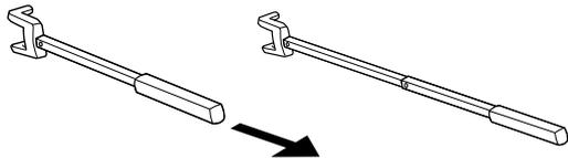
3. Pull up the screen slowly at a certain height using the Lifting Handle then grasp the Slat handle and raise the screen slowly keeping the slat level as you raise the screen.
