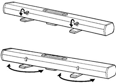
**Note:** Before carrying the case, rotate the feet, so they are out of the way.
