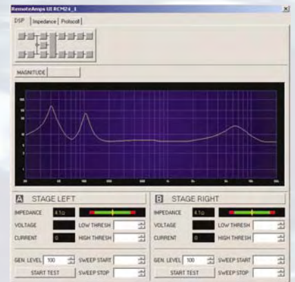
Supervision for each connected loudspeaker with individual upper and lower thresholds for impedance values. An out-of-limit device will show up immediately.
