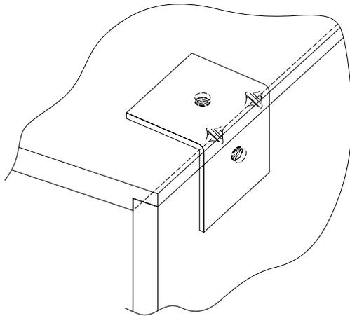
*The FRi Series features internal heavy gauge steel reinforcing brackets that are not only designed to provide high safety factor support for the 3/8-16 forged eyebolt rigging, but also to utilize the internal panels for each enclosure. These corner braces are required to maintain the structural integrity of the cabinet to performance levels listed in this manual.*
