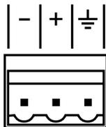
With an input sensitivity of 775 mV = 0 dBu and an input impedance of 20 k ohms, the electronically balanced inputs – INPUT CHANNEL A&B – are meant for the connection of control amplifiers, audio controllers, mixing consoles, etc.
