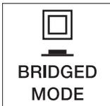
With the BRIDGED-MODE switch being engaged, using the channel A input for audio signal feed is mandatory, since input B provides no function. While the amplifier of channel A operates as usual, the audio signal is internally inverted and routed to the amplifier of channel B. Both amps – A and B – now work in push-pull operation to provide doubled output voltage at the BRIDGED-OUT connector.
