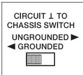
The ground-lift switch allows eliminating noise loops. If the power amplifier is operated together with other equipment in a 19" rack-shelf, setting the switch to its GROUNDED position is recommended. If the power amplifier is operated together with appliances with differing ground potentials, set the switch to its UNGROUNDED position.
