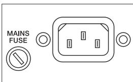
Under normal circumstances, the mains fuse only blows in case of fault. Replacing the fuse is only permissible when using a new fuse of the same type with identical amperage, voltage and blow characteristics. If the mains fuse blows more often, please contact an authorized service centre.
