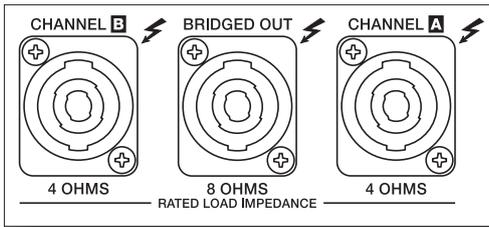
Power amp output connection for the two channels A (left) and B (right) is provided via SPEAKON-type output connectors.
