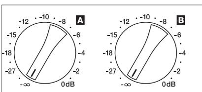
Detent potentiometers scaled in dB (steps of 1dB) for adjusting the power amp's overall volume. To prevent distortion in mixing consoles connected to your CP-Series amp, setting these controls to a value between 0dB and -6dB is generally recommended. The dB-scale provides direct indication of the control attenuation applied to the fixed internal amplification.
