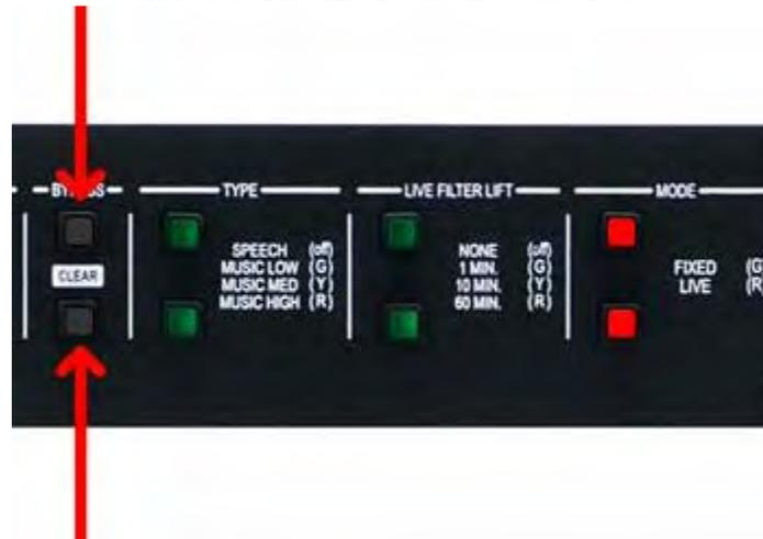
19. If you would like to lock the front panel (to prevent tampering), press and hold the channel 1 **LIVE FILTER LIFT** button. Hold this button until the filter LEDs flash all the way across (from the outside inward).
