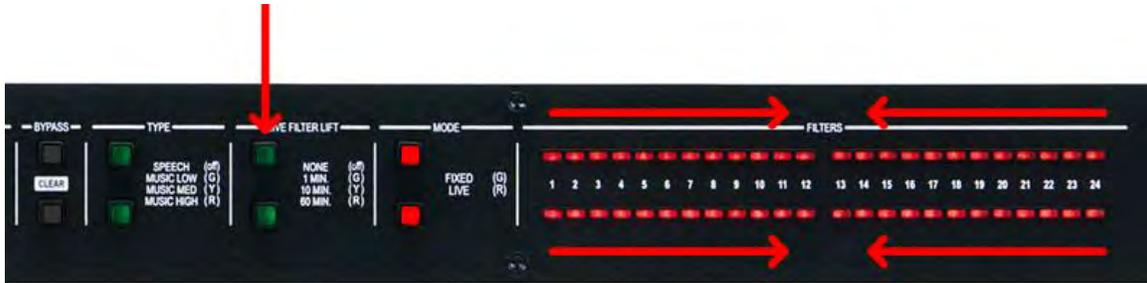
To unlock the front panel press and hold the channel 1 **LIVE FILTER LIFT** button until the filter LEDs flash all the way across (from the inside outwards).
