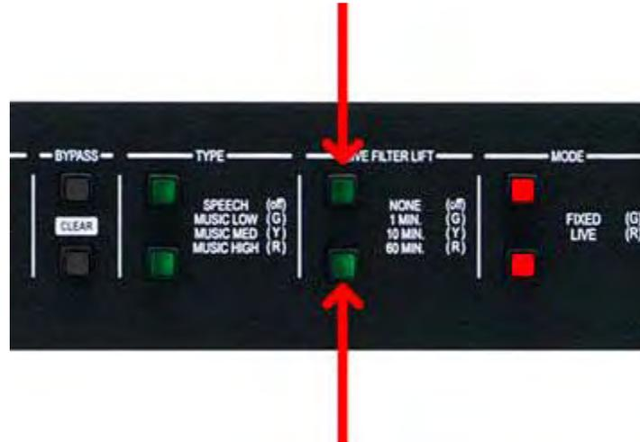
The AFS process is now complete. If, for whatever reason, you would like to restart the process, you can do so by clearing the filters and restarting with step 1. To clear all of the filters: Press and hold the BYPASS buttons until all lit filter LEDs begin to flash, now release. The filters are now cleared.
