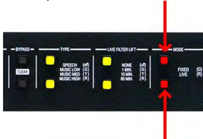
17. For a faster reaction time with the Live filters, try setting the filter **TYPE** to “Music Low” (green) or “Speech” (off).
