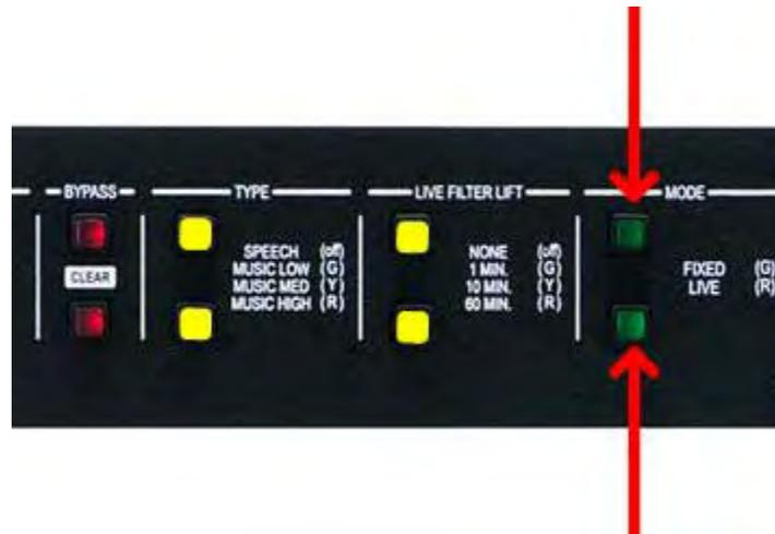
**14.** Disengage the Bypass buttons (LEDs off).
