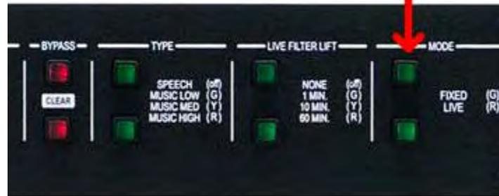
2. Hold this **MODE** button until the filter LEDs flash all the way across.
