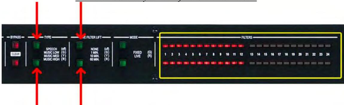
6. To exit the setup mode, press and hold the channel 1 **MODE** button. Hold this button until the filter LEDs flash all the way across.
