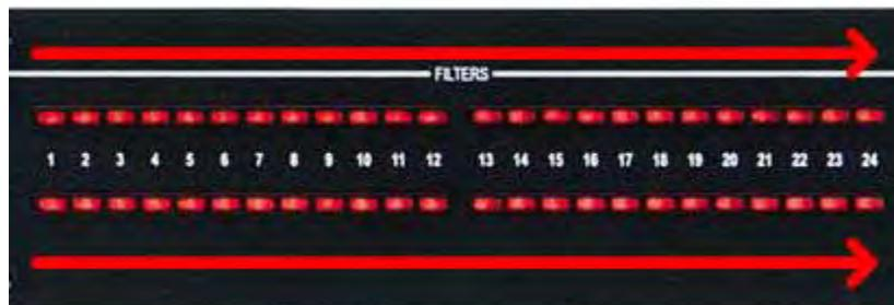
3. The Mode buttons should be lit a yellow or amber color. If they are not press each **MODE** button until they are both yellow. The filter LEDs will indicate how many total filters will be active.
